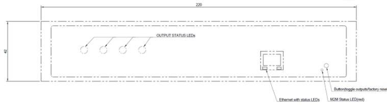
Figure 4 - PowerPDU 4PS front, dimensions [mm]
