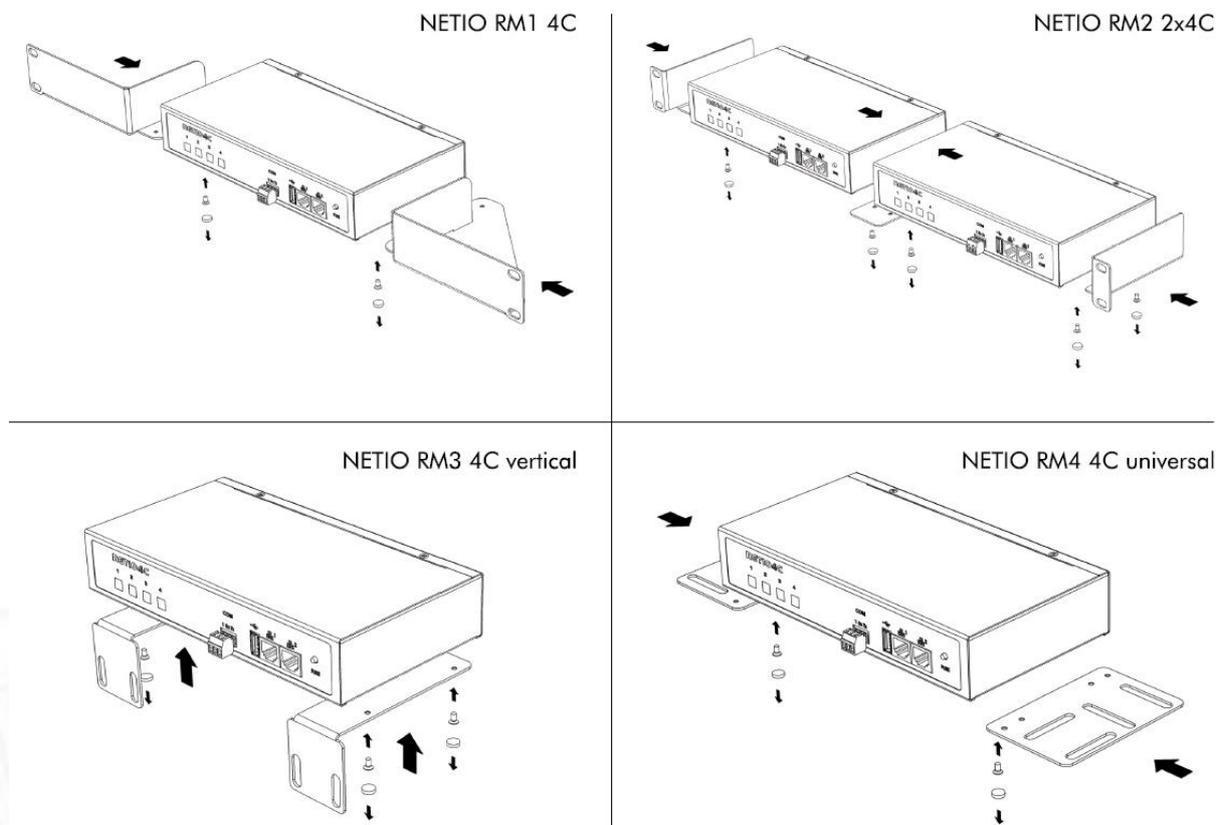
Figure 14 - NETIO RMx accessories for PowerPDU 4PS/4KS
