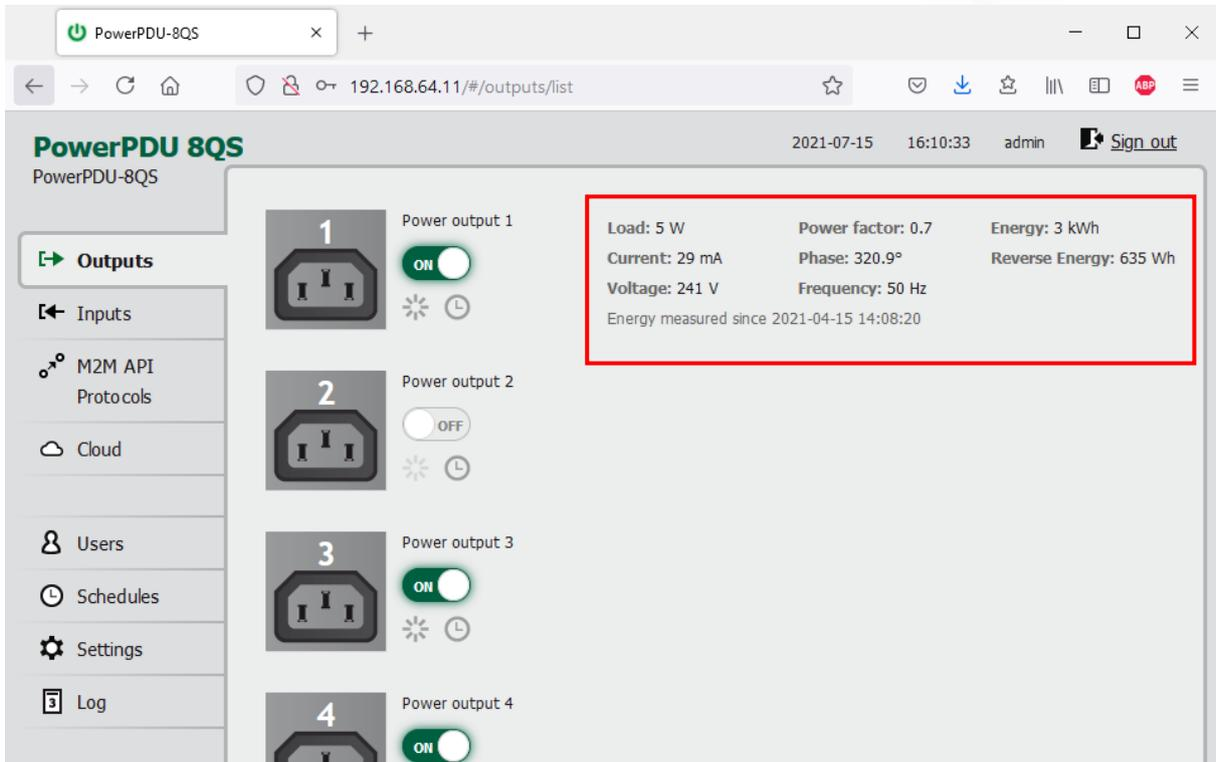
Figure 19 - Measured values - Output 1
