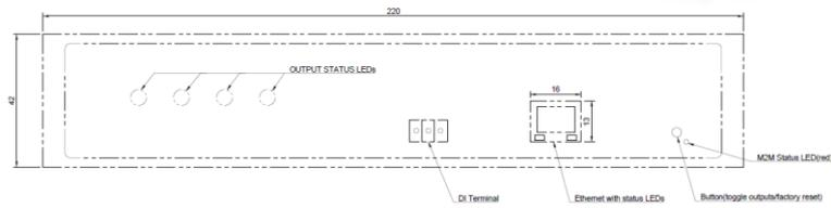
Figure 6 - PowerPDU 4KS front, dimensions [mm]
