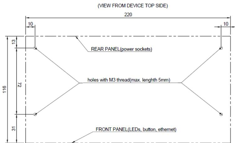
Figure 7 - PowerPDU 4KS - mounting holes for RM [mm]
