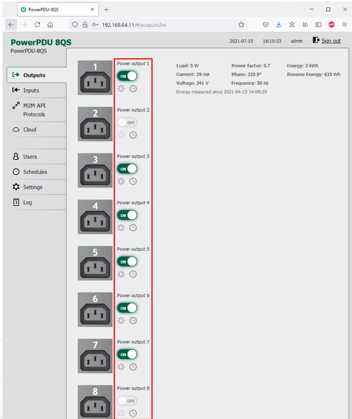
Figure 18 - Controlling the output
