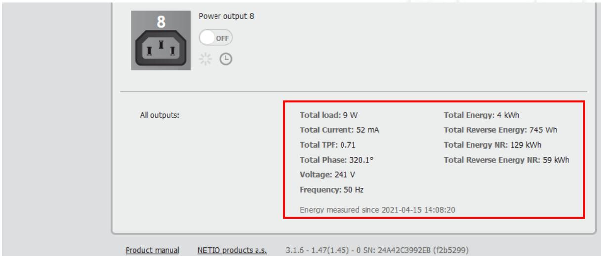
Figure 20 - Measured values - All outputs
