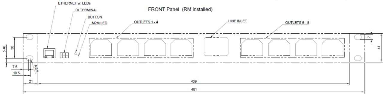
Figure 8 - PowerPDU 8QS - front, dimensions [mm]
