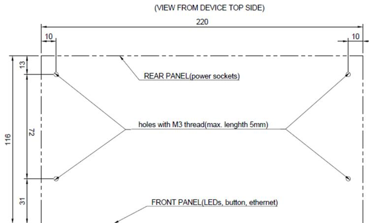
Figure 5 - PowerPDU 4PS - mounting holes for RM [mm]
